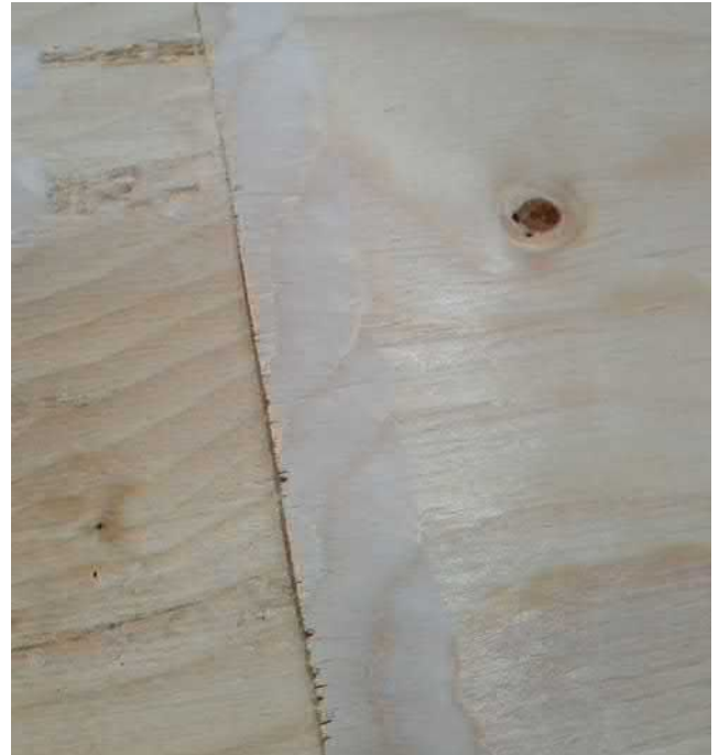
Figure1.37. Scarfed veneer end.
