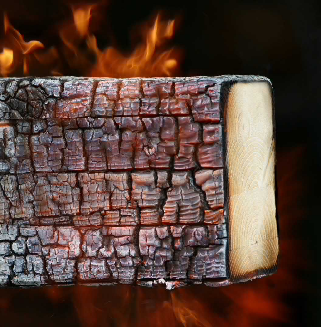
Figure 6.1. Charring of wood.
