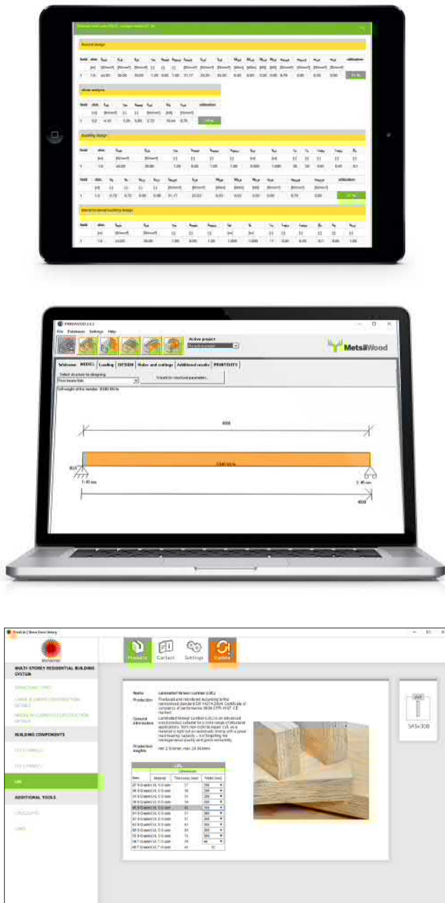
Figure 1.63. Design software for LVL structures: Calculatis by Stora Enso, Finnwood by Metsä Wood and portal of BIM objects by ProdLib.
