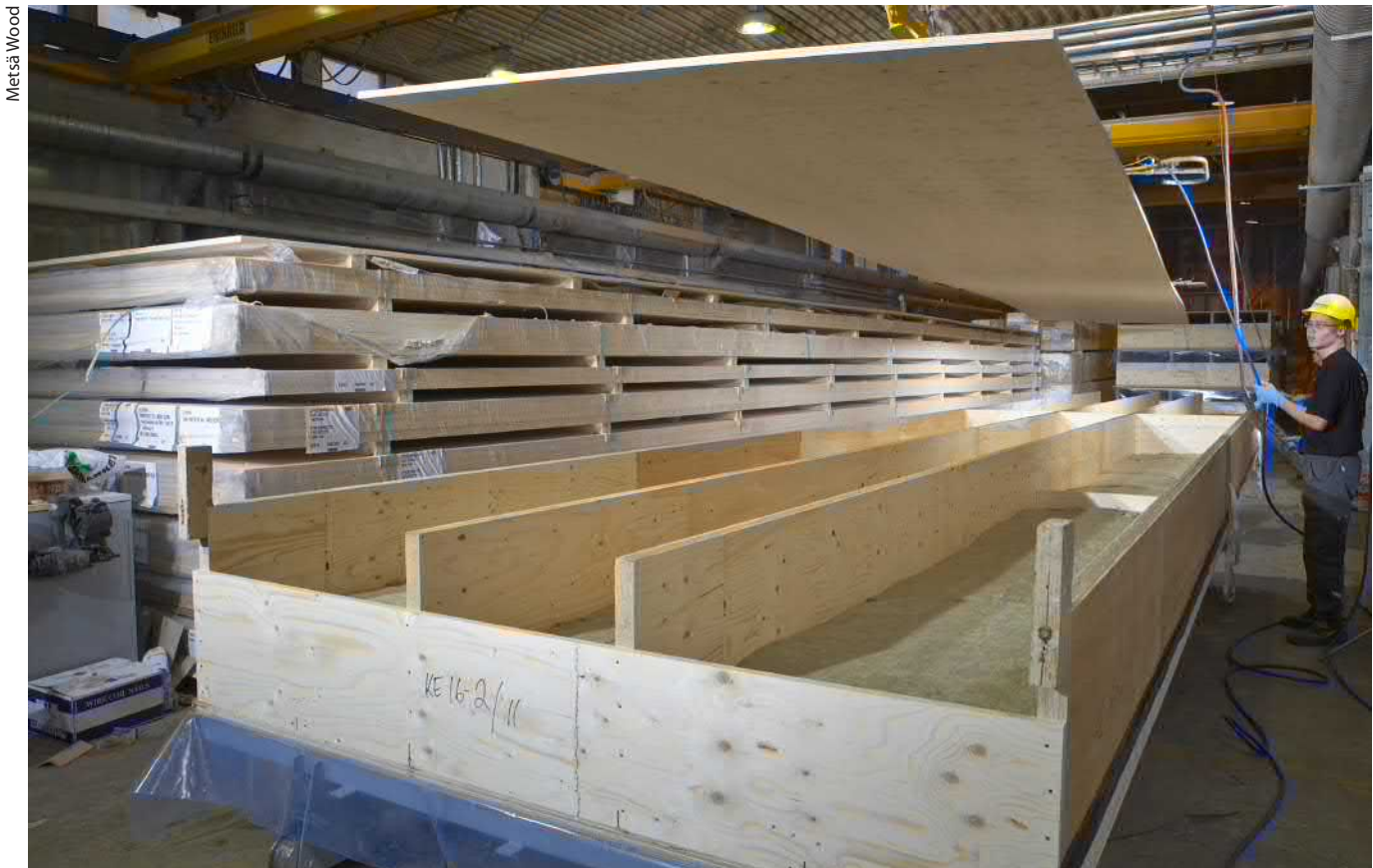
Figure 1.57: Manufacture of structurally glued LVL roof elements.
