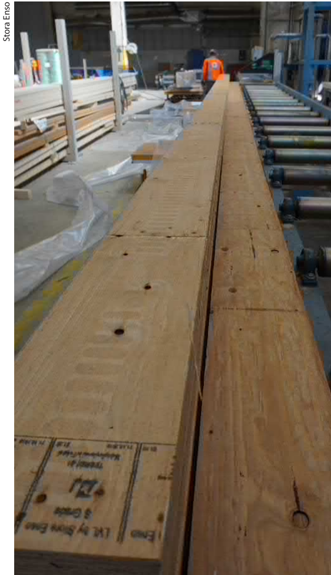
Figure 1.54. Moisture protection treatment of LVL-P beams by Stora Enso.
