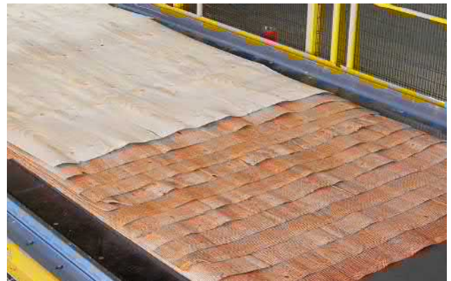
Figure1.40. Staggered layup ahead of the pre-press.
