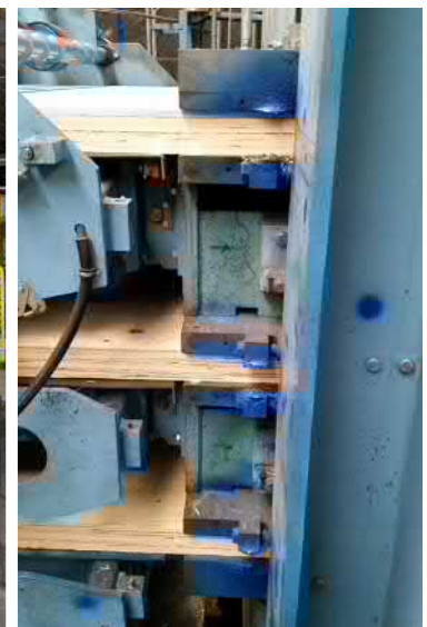
Figure 1.43. Feeding LVL billets into 3-level hot press.
