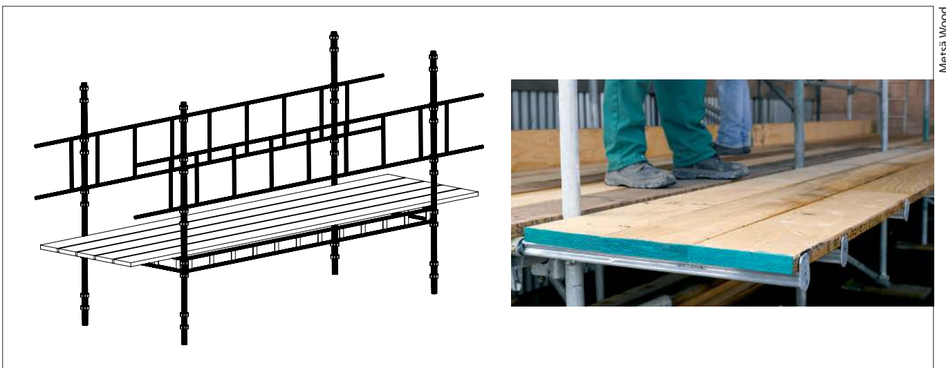
Figure 2.95. Scaffolding planks from LVL-P.
